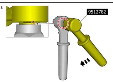
Use special tool: T9512782, Rivet nut tool
