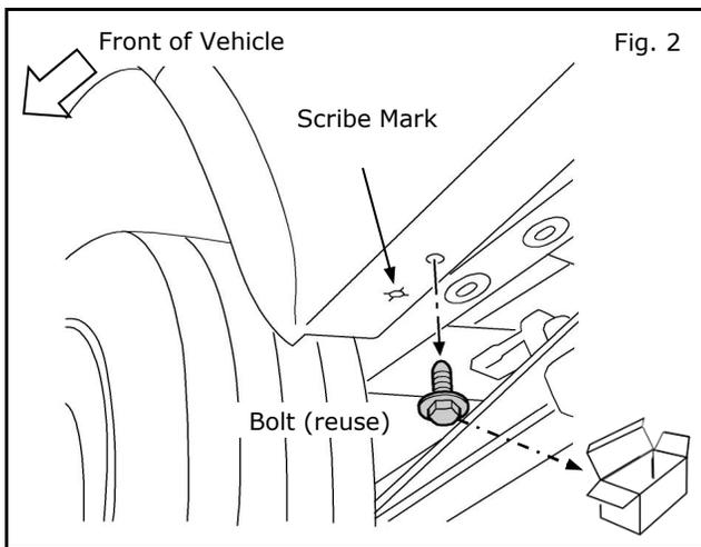
2) Remove bolt from bottom of rear bumper (keep to reuse).
