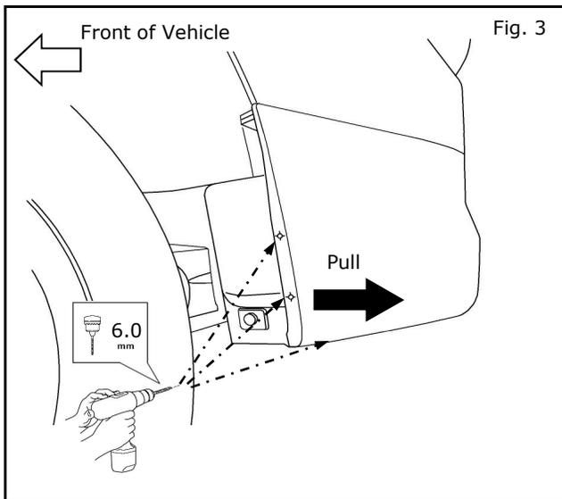
4) While pulling rear bumper outward, drill 6mm (1/4") holes at center of all scribe mark locations on bumper.
