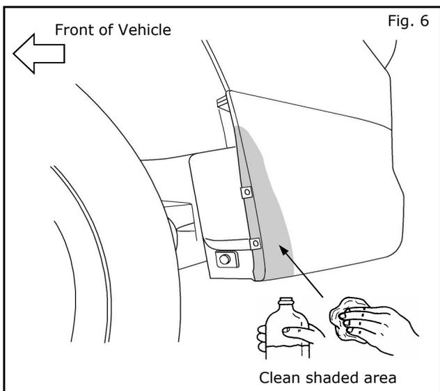
8) Clean installation surface (shaded area) with mild soap/water mixture.
