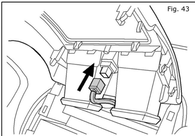
43. **Reconnect** two (2) electrical connectors behind the center stack upper trim panel
