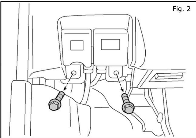
2. Remove two (2) 10mm bolts under the hood release lever. Remove the hood release lever assembly.
