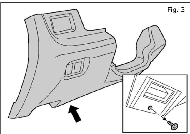
3. Remove one (1) phillips screw holding the diagnostic port to the panel.
