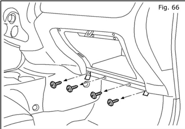
66. Remove four (4) Phillips screws from the bottom of the glovebox compartment.
