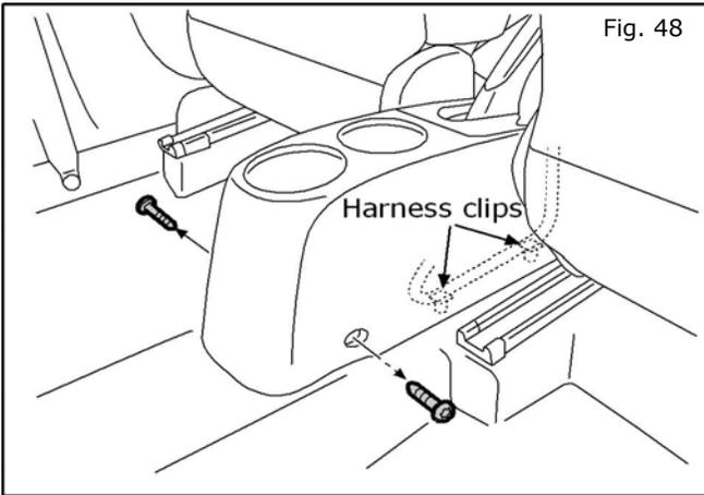
48. Remove two (2) T-20 Torx fasteners at the back of the center console on both sides.
