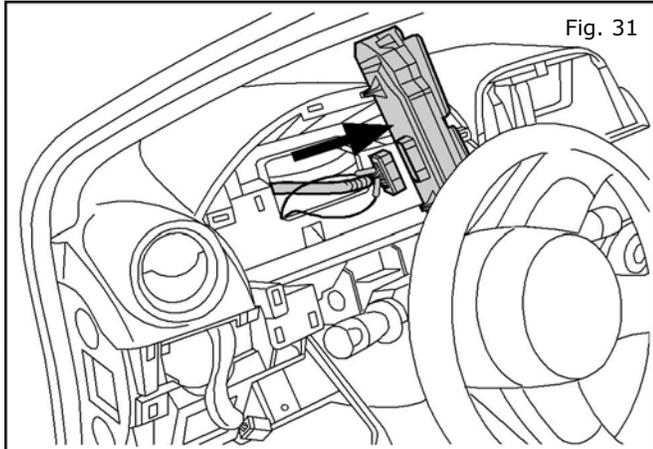
31. **Reconnect** the white electrical connector at the back of the instrument cluster.
