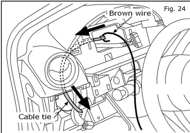
24. Use a long cable tie to feed the **Brown** accessory wire through the BCM opening and out the dash opening under the vent as shown.
