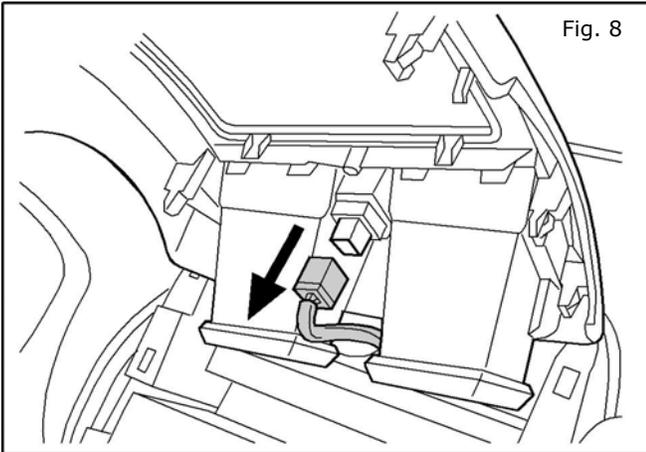
8. Disconnect two (2) electrical connectors behind trim panel and set panel aside.
