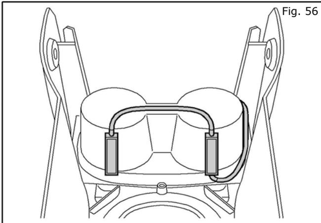
56. Clean the light stick mounting area with alcohol. Remove the pull tabs over the tape on the end cup holder light stick. Place the light stick over the black lens retainer as shown.
