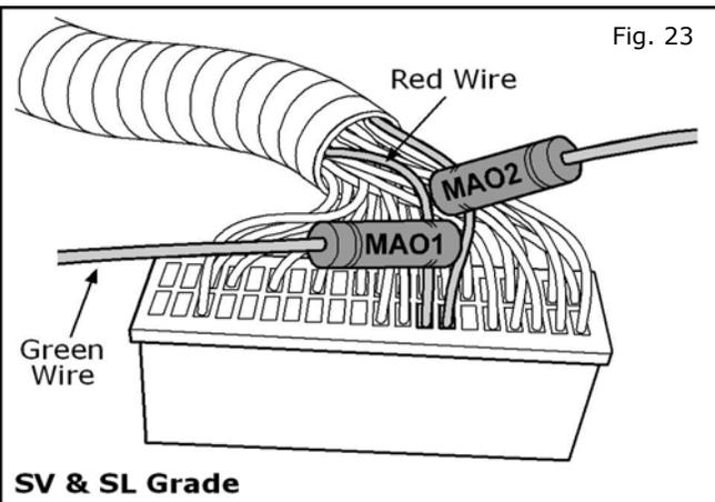
23. Use a Posi-tap and instructions to connect the **Green** wire from the accessory harness to the **Red** wire at the connector.
