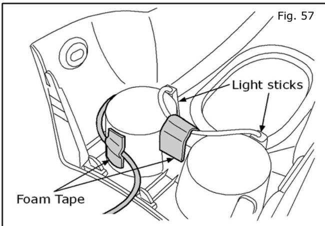
57. Secure excess wiring with foam tape as shown.
