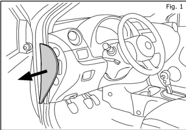
1. Carefully remove the LH Instrument side mask by the driver's door.
