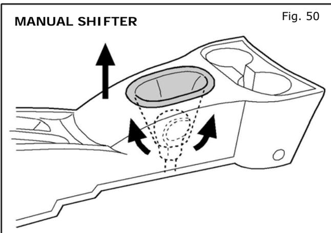
50. If vehicle is equipped with **manual** shifter, remove the shifter boot by carefully stretching the elastic collar up over the shift knob.
