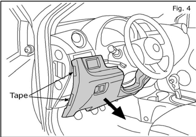
4. Carefully pull the steering finisher down away from the instrument panel. Pry the left side away first, then the right side.
