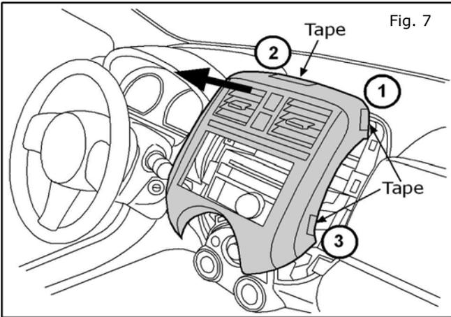
7. Carefully pry off center stack upper trim panel. Follow the pry off sequence 1, 2 and 3 as shown.
