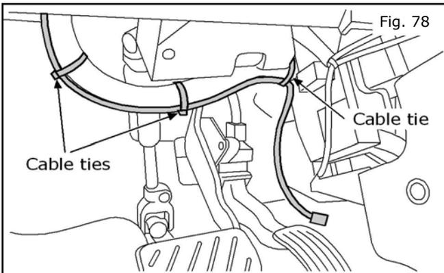
78. Secure the harness under the dash with cable ties as shown.
