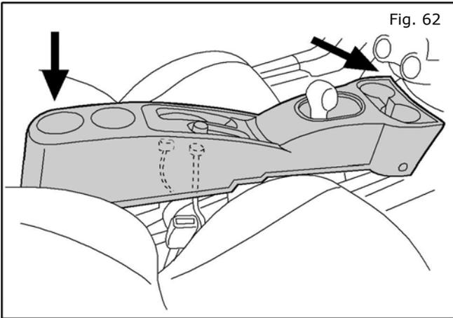
62. Once the console has cleared the parking brake and shifter, pull back and set the console over the two rear retaining screw locations.
