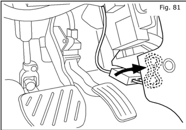
81. Stow excess wire bundle behind center stack finishing panel.
