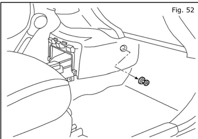
52. Remove two (2) plastic clip fasteners on either side of the center stack bottom finisher panel.
