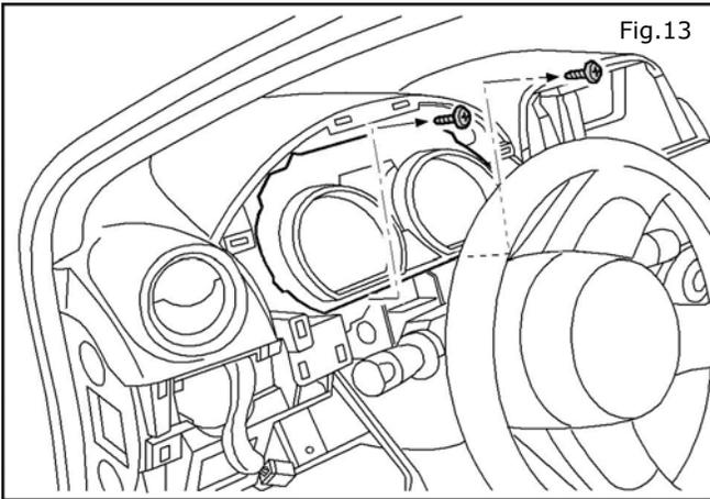
13. Remove two (2) Phillips screws at the bottom of the instrument cluster.
