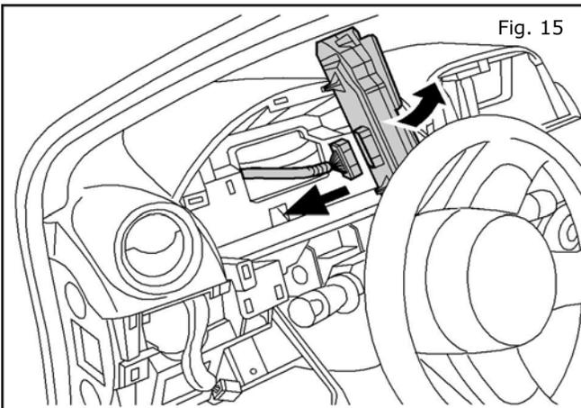
15. Rotate the instrument cluster upward and disconnect the white electrical connector from the back. Set the instrument cluster aside.
