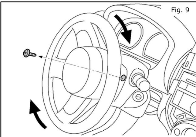
**NOTE: Turn the car ignition "On" and rotate steering wheel 90 degrees to the right.**
