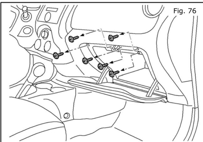
76. Install six (6) screws in the upper half of the glovebox compartment.
