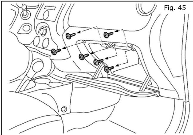
45. Open the glovebox door. Remove four (6) screws from the upper half of the glovebox compartment as shown.
