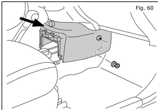
60. **Reinstall** the center stack bottom finisher panel. Once aligned, **install** two (2) plastic clip fasteners on either side.
