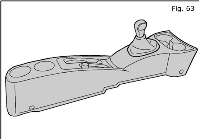
63. If vehicle is equipped with **manual** shifter, **reinstall** the shifter boot by carefully stretching the elastic collar down over the shift knob.
