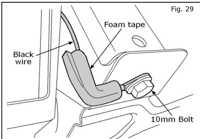
29. Remove one (1) 10mm bolt on the left side of the knee bolster bracket under the steering column. Place the bolt through the eyelet on the Black accessory wire for ground. Reinstall the bolt.
