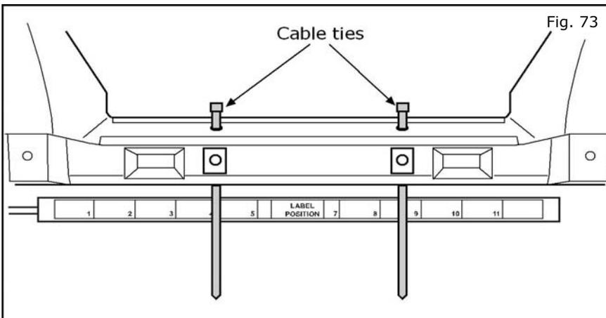
73. On the passenger side, Insert a cable tie in each mounting hole as shown.
