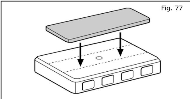
**NOTE: Attach one (1) 58mm x 82mm foam tape to the underside of the accessory control module, covering the screw in the center.**
