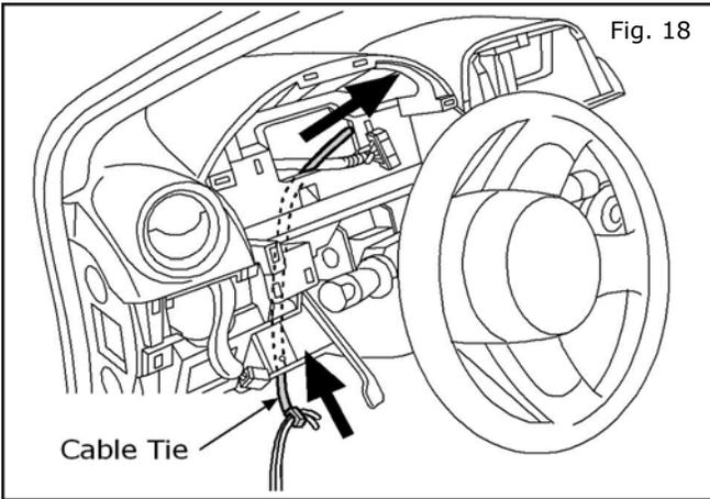
18. Push the ends of (2) wires, green and blue, through the end of a 15 inch cable tie and use the tie to direct the wires up through the dash to the BCM opening.
