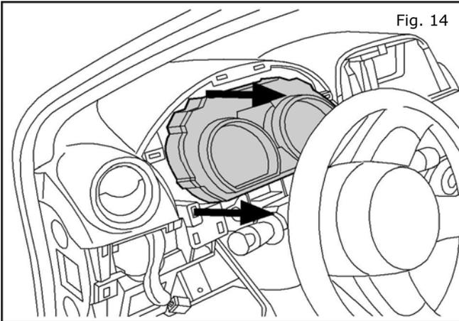
14. Remove the cluster by pulling it straight out to disconnect the clips at the top of the assembly.
