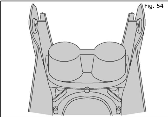
54. Place center console assembly upside down on work surface. Be careful not to scratch the surface.
