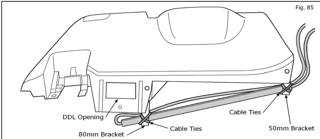
86. Pull the tape covers from the two (2) pieces of foam tape attached to the driver side light stick. Place the light stick over the "L" brackets with the LEDs pointing down such that the tape rests on the 'L' bracket. Secure each location with two (2) 4 inch cable ties.
