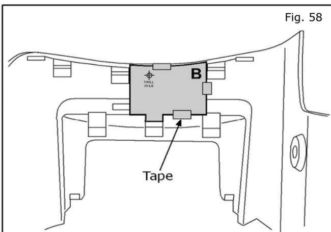
58. Place center stack bottom finisher panel face down on work surface. Be careful not to scratch the surface.
