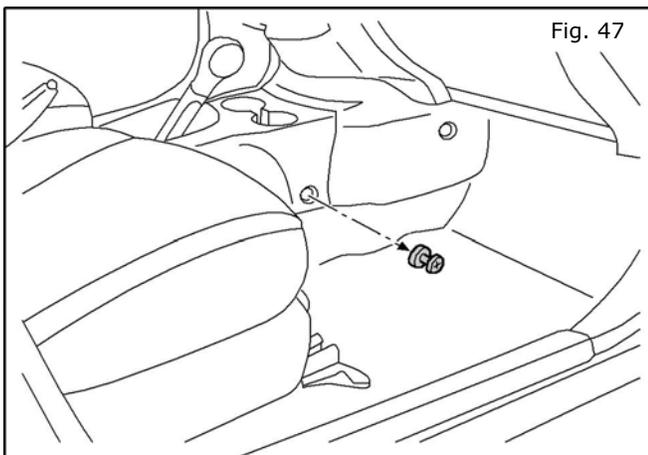
47. Remove two (2) plastic clip fasteners on either side of the center console.
