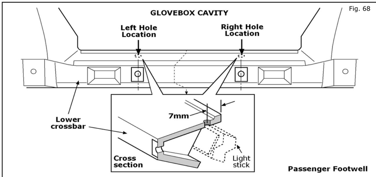
68. Prepare to mark drill locations at the glovebox opening. Measure and mark in from the back edge, 7mm. Mark the left and right mounting holes centered in alignment with the two existing holes on the lower cross bar as shown.
