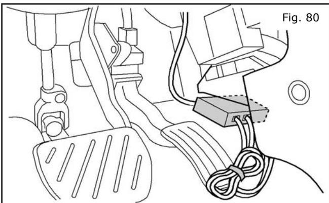
80. Peel the cover off the tape on the controller and place the controller on the carpet under the center stack.
