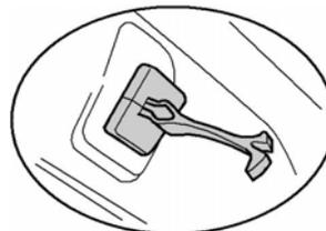
**DO NOT REUSE THE CLIPS THAT WERE REMOVED EARLIER. INSTALL THE NEW CLIPS PROVIDED IN THE KIT.**
