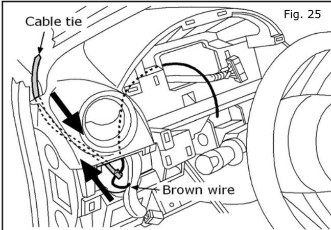
25. Feed a 15 inch cable tie down through the dash from the A Pillar. Push the ends of the **Brown** wire through the end and use the tie to direct the wires up through the dash to the A Pillar.
