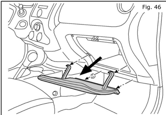
46. Press down **firmly** on the glovebox door side supports to release them and then unsnap the door from the lower hinge.
