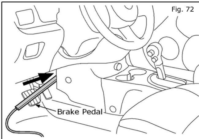
72. Push the passenger light stick through the center stack to the passenger footwell. This is the light stick with the loop.
