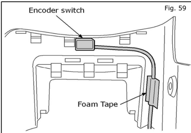
59. **Install** the encoder so that the shaft is outside the front of the finisher panel.
