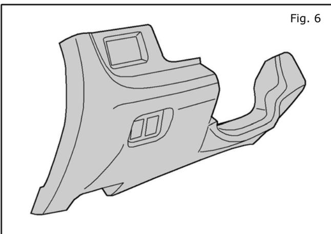
6. Remove the steering finisher and set aside.
