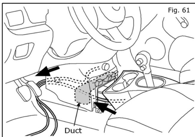
61. Carefully place the modified center console into the car. Position the console over the parking brake and shifter by gently moving the console forward as it is lowered.
