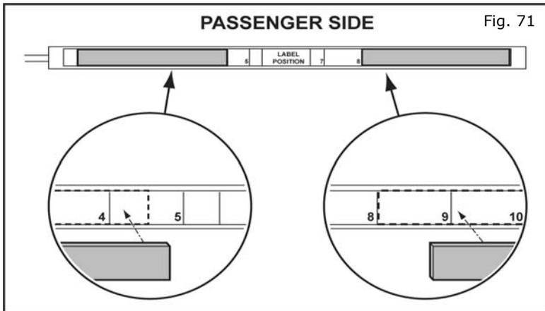
71. Prepare the passenger side light stick. Clean the Non- LED areas with alcohol wipe. Fix the long **12.5mm X 100mm X .7mm** piece of double sided foam tape at location **0.5 to 4.5** AND at location **8 to the END**.
