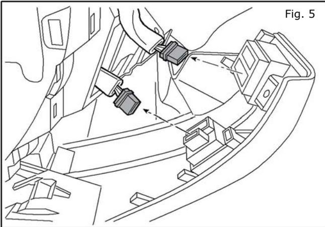
5. Disconnect two (2) electrical connectors from back of panel.
