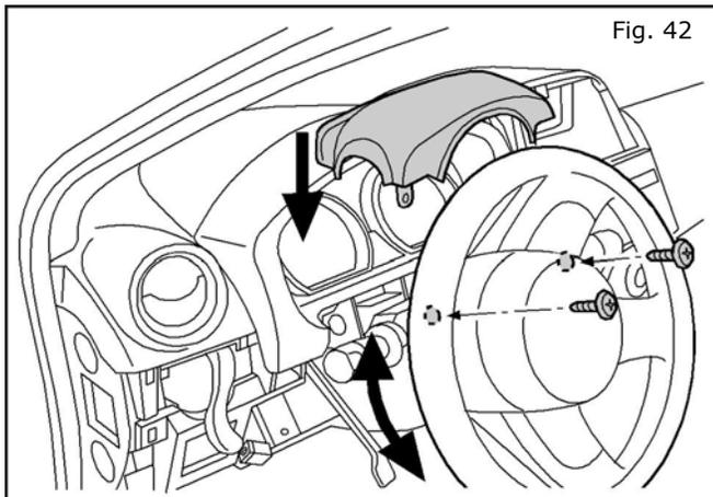
42. **Reinstall** the trim panel on the top half of the steering column
