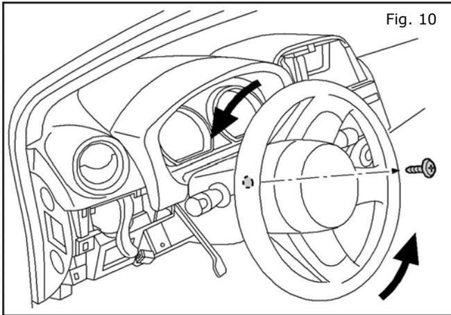
**NOTE: Rotate steering wheel 180° in the opposite direction**
