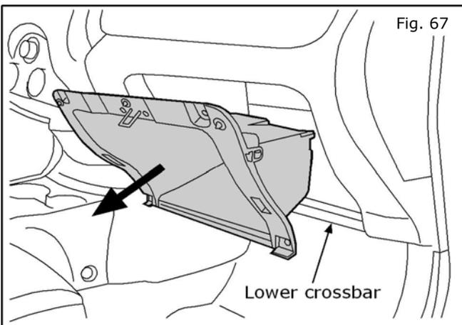
67. Grip the door latch loop and pull down and outward to remove the glovebox compartment.
