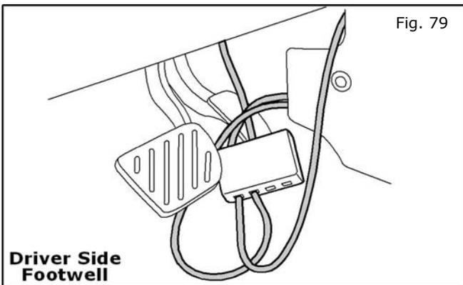
79. Route accessory harnesses under the center stack. Plug the accessory harnesses into the control module and allow to sit under center stack.
