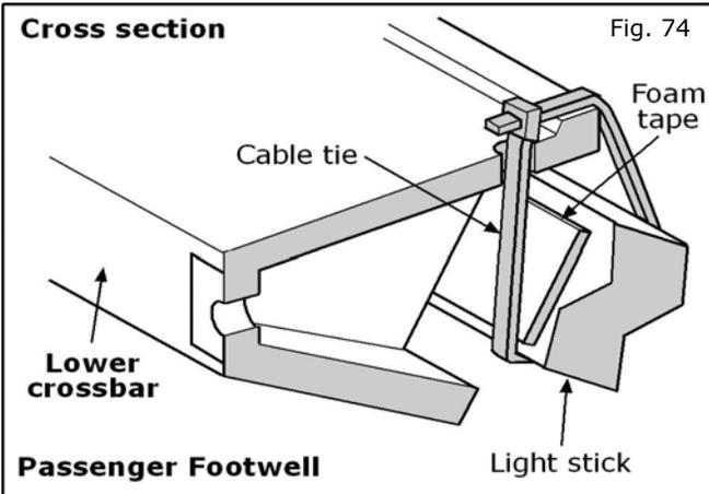
74. Pull the tape covers from the two (2) pieces of foam tape attached to the passenger light stick. Place the light stick behind the lower glovebox cross bar with the LEDs pointing down. Secure each the light bar with with three (3) 4 inch cable ties at the drilled holes locations.
