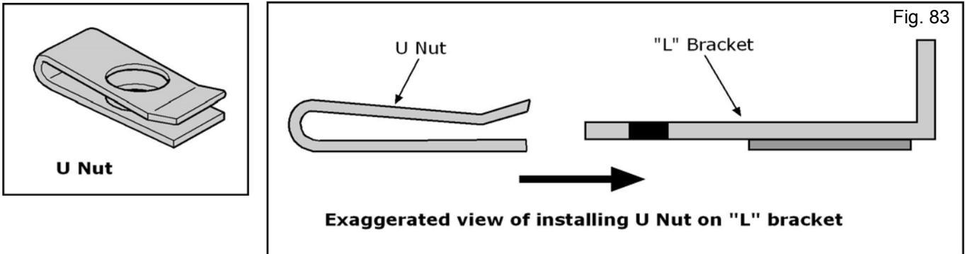
84. Attach the two (2) "L" brackets with U nuts to the inside of the steering finisher with two (2) phillips screws. The 80mm bracket will be next to the DDL opening.
