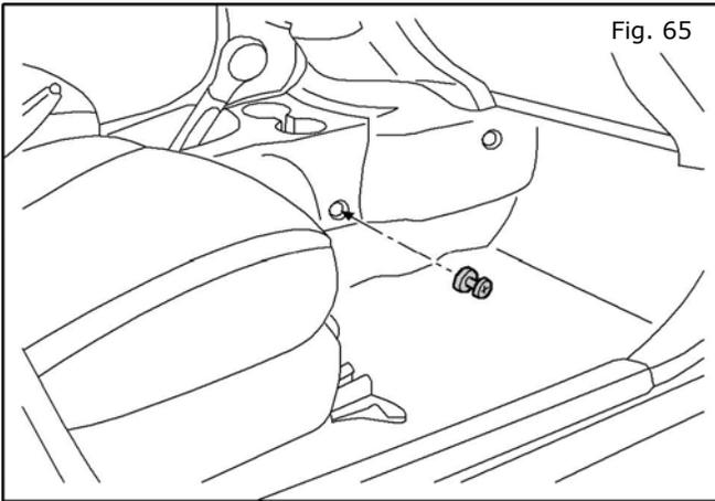
65. **Reinstall** two (2) plastic clip fasteners on either side of the center console.
