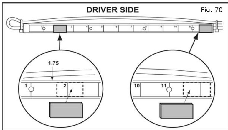
70. Prepare the driver side light stick. Clean the LED areas with alcohol wipe. Fix the short 12.5mm X 19mm X .7mm piece of double sided foam tape at location 1.75 to 2.5 AND at location 11.5 to END.
