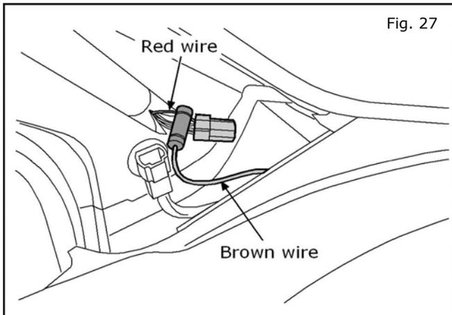
27. Using a Posi-Tap, connect the **Brown** wire from the accessory harness to the **Red** wire at the connector.
