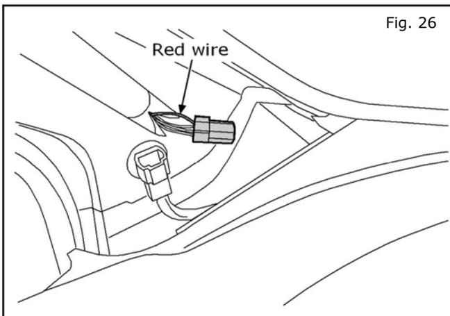
26. Disconnect the electrical connector at the bottom of the A-pillar.
