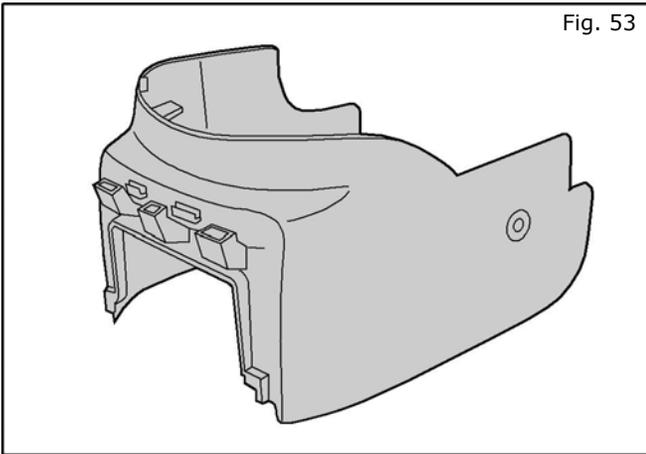
53. Remove the center stack bottom finisher panel and set aside.
