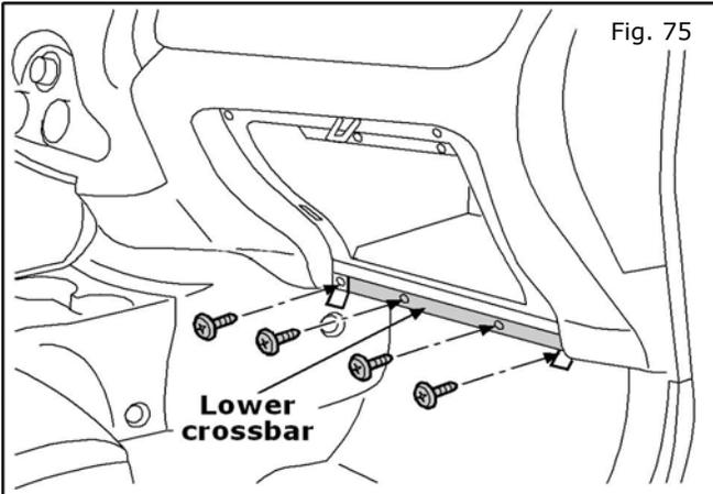
75. **Reinstall** the glovebox compartment. Install four (4) phillips screws in the bottom of the glovebox compartment.
