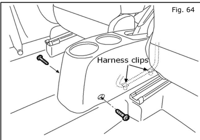
64. Reinstall two (2) harness clips at metal studs. **Reinstall** two (2) T-20 Torx fasteners at the back of the center console on both sides.
