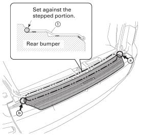
3) Place the Rear Bumper Plate (1) on the rear bumper. Set the front end of the Rear Bumper Plate (1) against the stepped portion of the rear bumper. Then adjust the clearances @ and b to be even.
