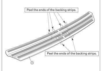
2) Peel off the ends of the backing strips from the adhesive tapes at the back of the Rear Bumper Plate 1).
