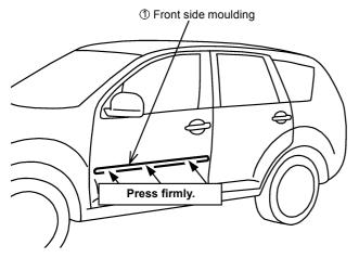
7) Press the adhesive tape portions of the front side moulding ① firmly. Remove the cardboard.
