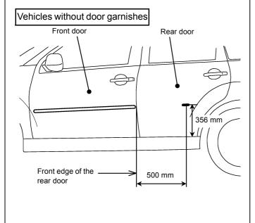
1) Mark the one positions shown in the drawing with the water-soluble felt pen for reference only.
