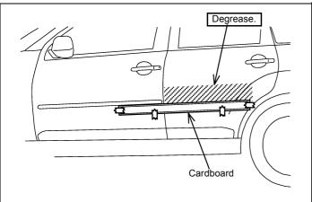
2) Wipe clean and degrease the surface to attach the rear side moulding ② (hatched portion in the drawing) using a clean shop towel moistened with isopropyl alcohol or degreaser.
