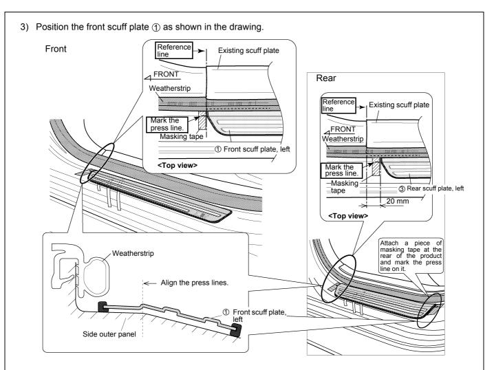
Adjust the position of the front scuff plate ① so that it is parallel with the vehicle's existing scuff plate. Then slowly peel off the backing strips in the order of 1 to 3. After that, press the front scuff plate ① firmly from the front to the rear to fix it securely.
