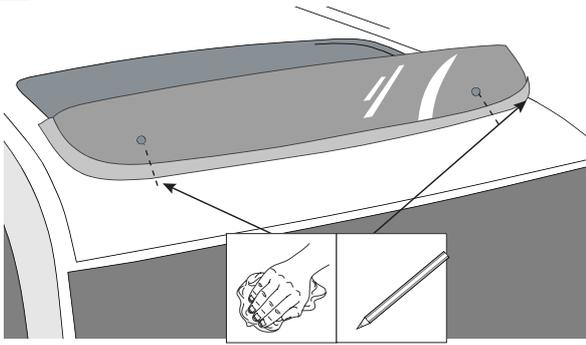
Open the sunroof and clean installation areas thoroughly. Trial fit Sunroof Deflector centrally on roof. Take note and mark the areas on Sunroof Deflector where rubber extrusion and metal clips are to be positioned. Remove Sunroof Deflector.
