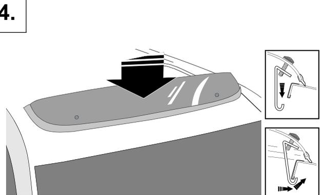
Re-fit the Sunroof Deflector centrally on the roof. Position clips at front of the sunroof opening. Depress the corners of the Sunroof Deflector to hook the clips under the inside edge of the opening.
