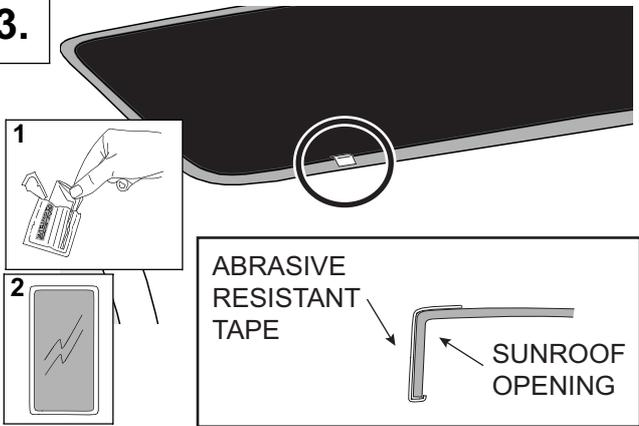
At the previously marked clip positions, clean the sunroof opening with alcohol wipe provided, remove any residue with a dry clean cloth. Adhere abrasive resistant tape at the contact areas of the inner flange area of the sunroof opening, as shown.
