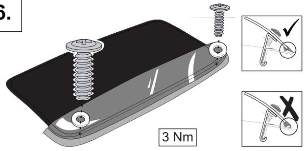
Ensure rubber seal is spread out flat against the roof and does not curl under at any point. Tighten the screws, alternating between sides, until the clips seat against the Deflector. **DO NOT OVER TIGHTEN!**
