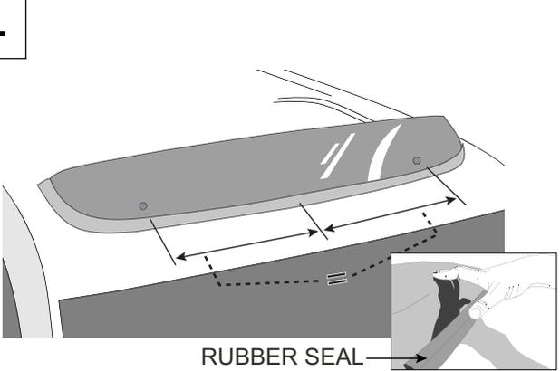
Before tightening, make sure the Sunroof Deflector is centered on the roof and that the clips are seated correctly and over the abrasive resistant tape.
