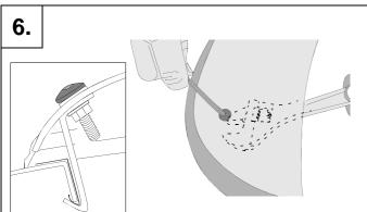
Using an allen key and a wrench, start to tighten one end while at the same time applying pressure to the top front corner near the screw to ensure the rubber gasket is flat against the roof and not curling under itself. Repeat process to the other side.
