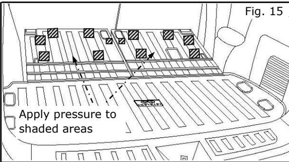
20) Apply pressure to shaded areas in figure 15 to secure hook and loop features.
