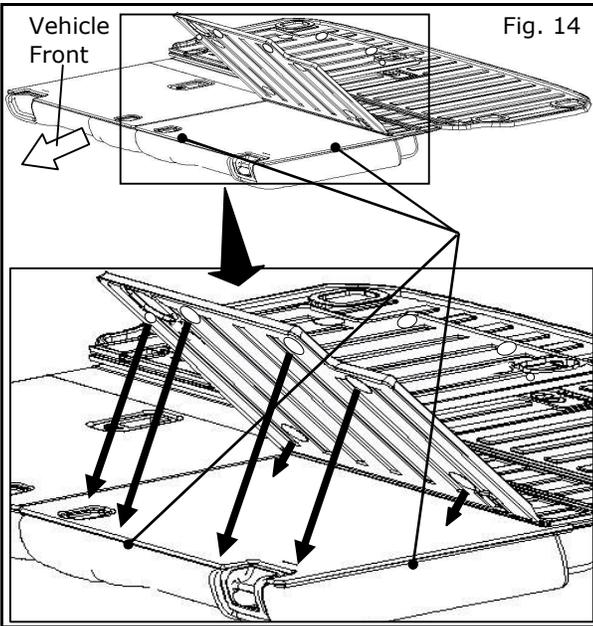
18) Unfold driver side protector flap and align edges and openings to seat back edges and features.
