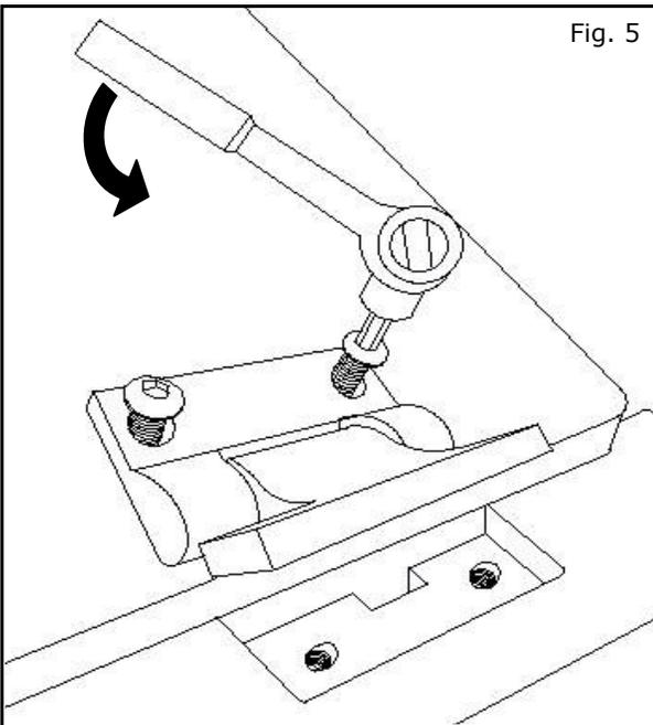
6) Loosen and remove (2) passenger side hinge screws with 4mm allen head socket driver. Keep screws for later use. Discard hinge.
