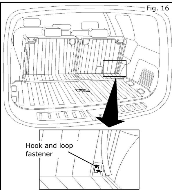
21) Pull seat straps to return seats to original position and re-attach seat straps to hook and loop fasteners.
