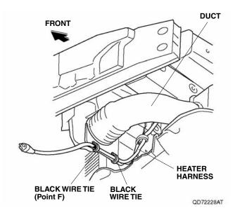
30. Secure the heater harness to the duct with one black wire tie at the white mark (point F).
