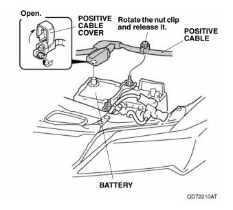
7. Remove the battery, the plate, and the covers.
