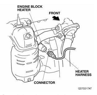
Secure the heater harness to the thermostat case with one brown wire tie at the white mark (point A).
