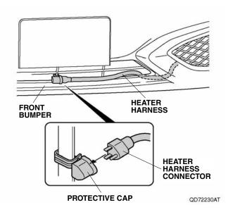
33. Secure the heater harness to the front bumper with a black wire tie.
