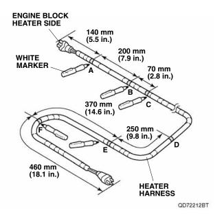
9. Install one wire tie with clip to the heater harness at point E.
