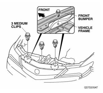
Remove the two self-tapping screws, two bolts, two short clips, and twelve medium clips.
