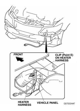
26. Secure the heater harness to the vehicle panel with a black wire tie.
