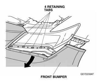
With the help of an assistant, remove the front bumper and unplug the vehicle connector. Place the front bumper on a blanket to prevent damage.
