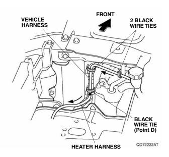
23. Secure the heater harness to the vehicle harness with a black wire tie at the white mark (point D).
