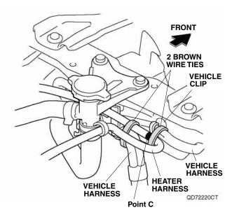
19. Secure the heater harness to the vehicle harness with one brown wire tie.
