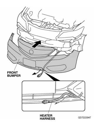
32. Attach the protective cap to the front bumper, and plug the heater harness connector into the protective cap.
