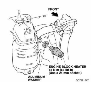
14. Plug the connector end of the heater harness into the engine block heater. Make sure the heater harness connector is fully seated in the engine block heater.
