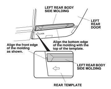
12. Press on the left rear body side molding firmly with the palm of your hand while removing the adhesive backings. Remove about 2 to 4 inches at a time.
