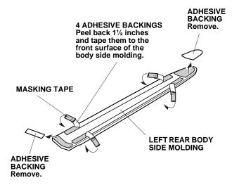
11. Align the edges of the left rear body side molding with the edges of the rear template as shown, and install the left rear body side molding on the left rear door.
