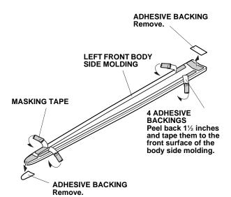
Align the edges of the left front body side molding with the edges of the front template as shown, and install the left front body side molding on the left front door.
