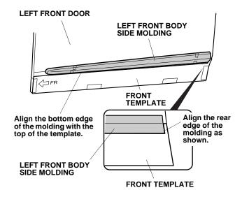
5. Press on the left front body side molding firmly with the palm of your hand while removing the adhesive backings. Remove about 2 to 4 inches at a time.
