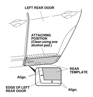
9. Clean the door surface where the left rear body side molding will attach using one alcohol pad. Allow the alcohol to dry.
