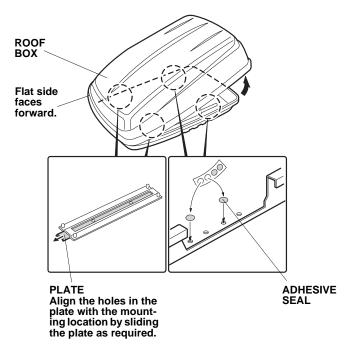
Attach an adhesive seal over each of the four unused mounting holes (two on each side) at the rear of the base of the box. The seals will help prevent water from entering the roof box. Then, remove the roof box from the crossbars. 4. Using isopropyl alcohol on a shop towel, clean four brackets B where the small pads will attach. Remove the adhesive backings from the small pads, and attach them to the brackets B.
